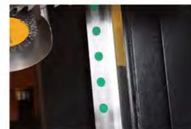
Applying high rigidity linear guide ways instead of vertical bars.
