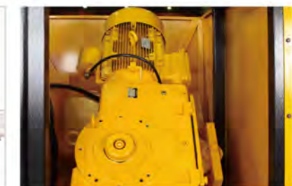
High torque Gearbox quietly powers the saw blade.
