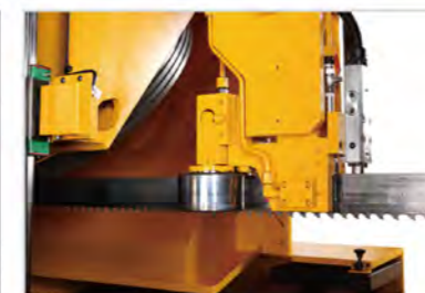
Automatic Blade Tracking Guide actuated by linear guide ways.
