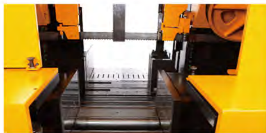
Automatic centering coolant supply unit cools down the cutting area directly.
